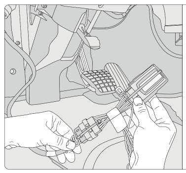
**5)** Ensure it is securely seated and use a zip tie to hold the connectors from separating.
