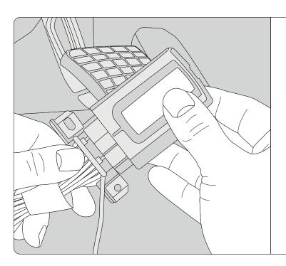
**4)** Connect the GO device to the receptacle side of the HRN-BD16S1.
