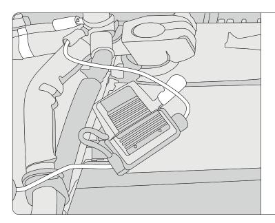
7) Locate the positive terminal of the battery. Make the connection between the positive terminal and the supplied (5A) fuse, ensuring the connections are corrosion protected. Fuse must be within 6" (150mm) of the terminal. Connect the Red wire from the HRN-BD16S1 to this fused connection to the battery.
