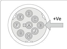
1) Confirm vehicle Master power switch is + positive switched. This is done by metering between the positive (J1939) pin and the chassis, and toggling the master power switch. If the vehicle is ground switched, the HRN-BD16S1 cannot be used.
