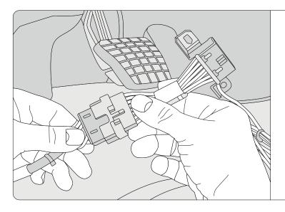
2) Connect the T-Harness 16 pin connector to the plug side of the HRN-BD16S1.
